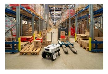
NVIDIA Nova Carter Robot powered by NVIDIA Isaac Perceptor & RGo Perception Engine running in a busy warehouse after very short integration and set-up of the facility
